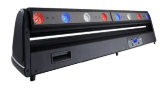
An array of individually controlled 15W RGBW LED modules equally spaced along the strip with fully adjustable zoom from 8-67 degrees. The strip itself has a very fast 270 degree tilt movement which can be precision indexed or programmed to produce rapid sweeping movements. Pre-programmed colour macros and pixel control makes this fixture quick and easy to programme. Tungsten lamp emulation and fade effects at 2700 K and 3200 K are included. Wireless technology CRMX is available as an option.
